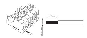
Use a small slotted screwdriver with downward force, embed the conductor as shown in the diagram
